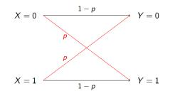
Figure 4: Binary Symmetric Channel
